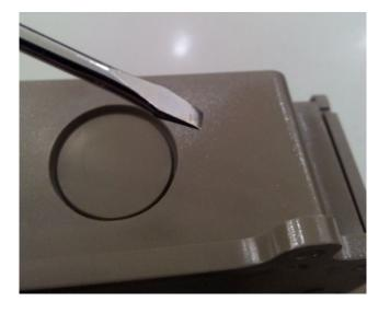
2. Using a slot screwdriver, aiming at the edge of the knockout, gently tap the screwdriver with a hammer until the screwdriver blade goes through.
